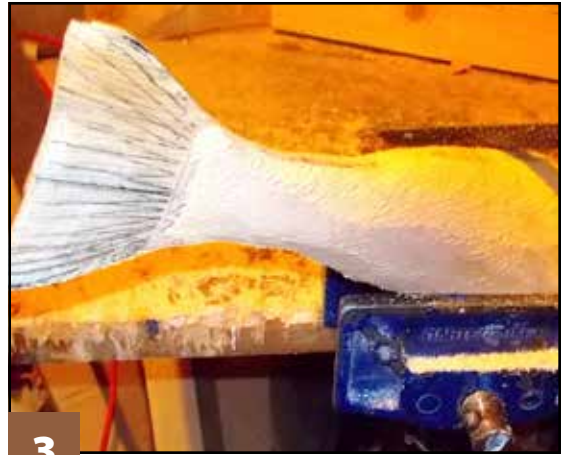
3 Round the body. Use a coarse rasp. Then, use the same tool to begin shaping the head.
