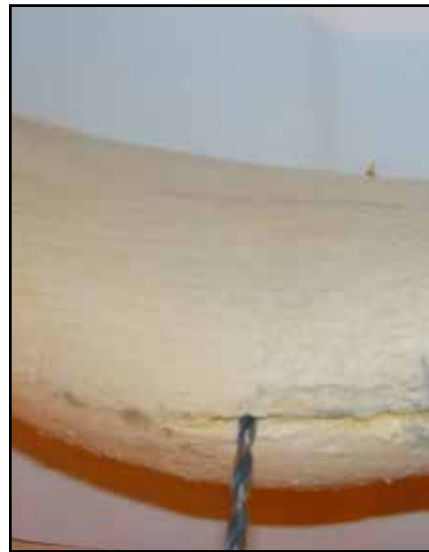
5 Drill holes for the pectoral fins. Use a hand drill with a \frac{1}{8} " (3mm)-diameter bit. Drill holes as close together as possible to create a \frac{1}{8} " (3mm)-deep slot about \frac{1}{2} " (13mm) long. Clean up the slot with a sharp chisel. Use the same process to create a \frac{1}{8} " (3mm)-deep by 2" (51mm)-long slot for the dorsal fin.
